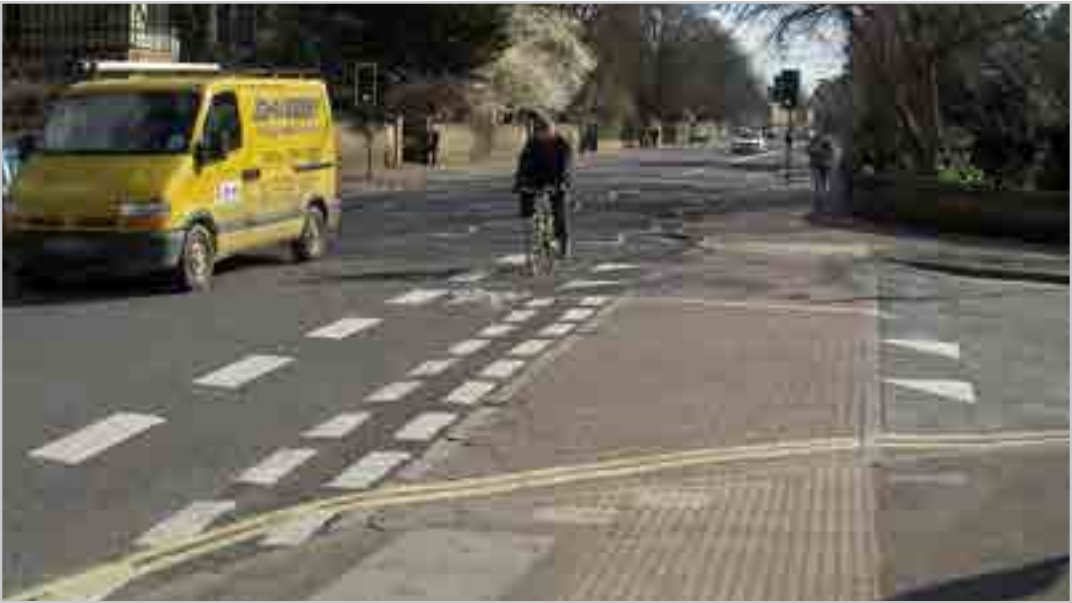
Raised table Raised tables at junctions reduce speeds of turning vehicles at side roads or across the entire junction.
