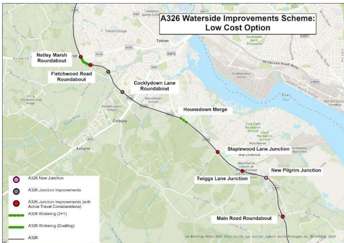
Figure 1-4: A326 Waterside Improvements Scheme – Low-Cost Option
