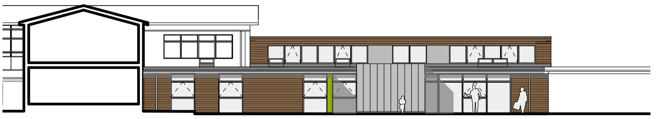
Existing Junior School Administration Main Entrance Library Existing Infant School Proposed North Elevation of New Link Entrance (1:250@A3)
