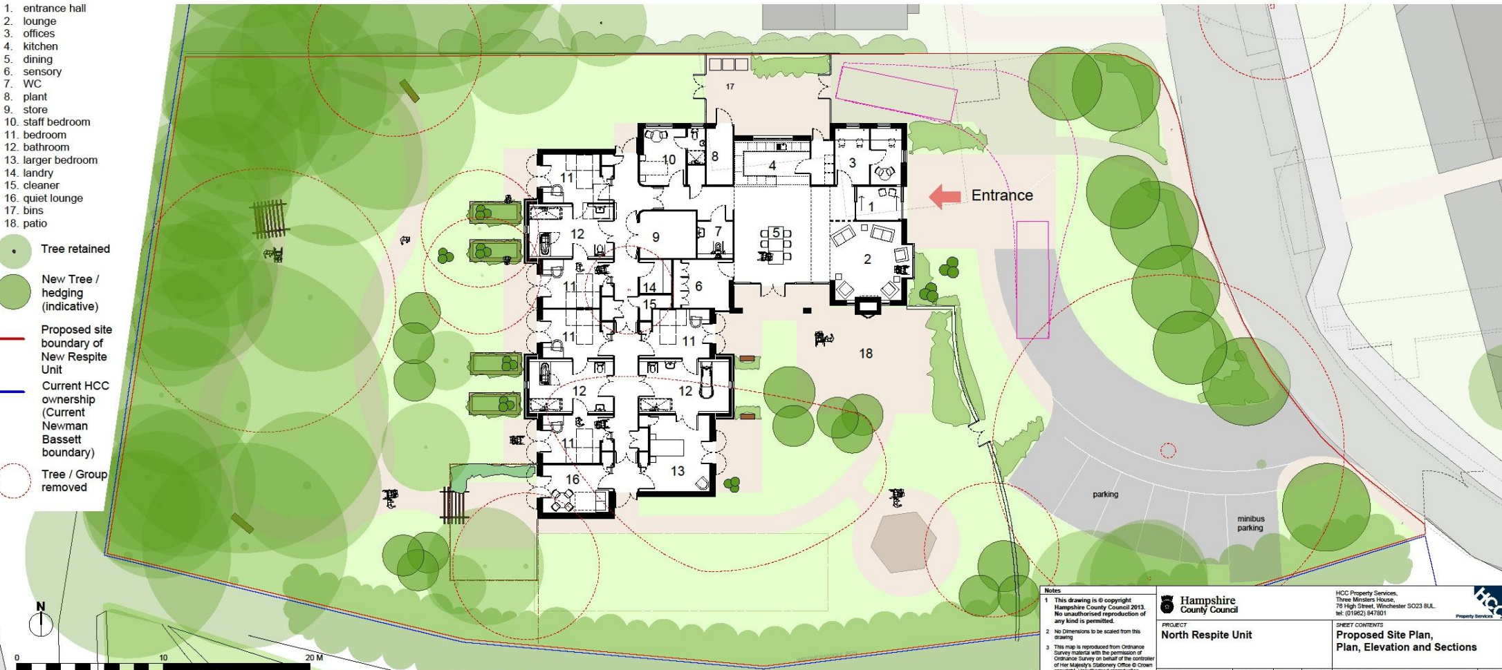
Ground Floor Plan and External Works at 1:125
