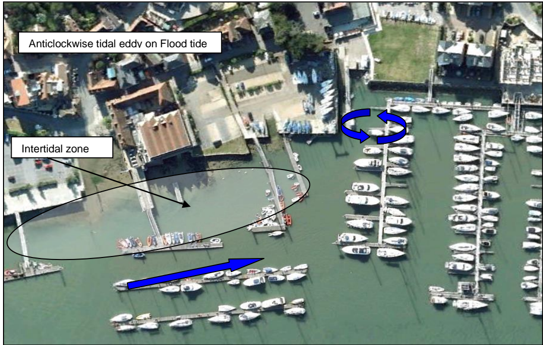
Figure 7.5 Flood Tidal Flows & Resultant Anticlockwise Eddy
