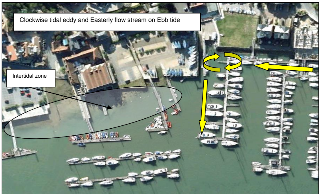
Figure 7.6 Ebb Tidal Flows & Resultant Clockwise Eddy & Easterly Flow Stream
