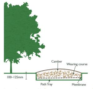
Lay wearing course: 100-125mm depth of compacted material (usually scalpings or natural stone aggregate), extending over edges of path tray.
