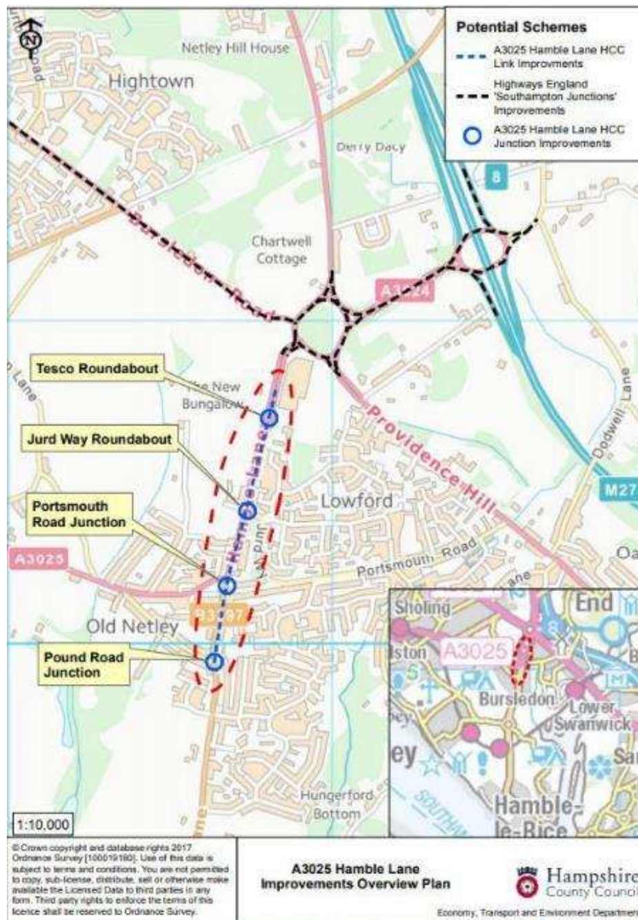
Figure 6: Plan of the Hamble Lane North Improvements Scheme that was previously consulted on
